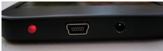
The USB-mini connector on your camera should look like this.
